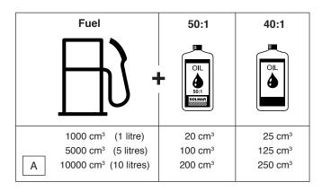
The brushcutter is powered by a high-performance two-stroke engine. The engine runs on a mixture of gasoline and two-stroke engine oil.
